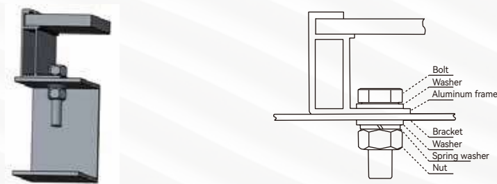
Figure 5 Bolt Installation of Mono-facial Modules
