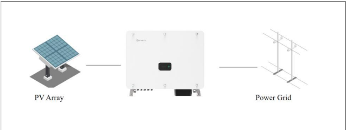
Figure 1-1 Composition of the PV power generation system
